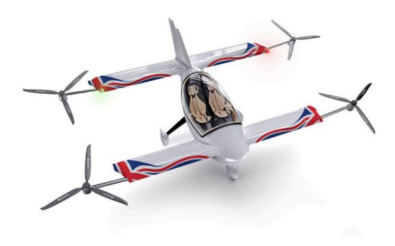
The Axe also offers greatly increased safety compared to a helicopter, thanks to its eight-motor distributed propulsion, each with its own power supply and its glide ability arising from its four wings, which enables power-off landing. Additionally, the Axe is fitted with a ballistic parachute - which a helicopter can never have due to the positioning of its rotors.
