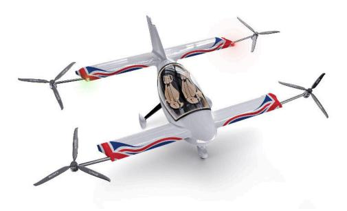
The Axe also offers greatly increased safety compared to a helicopter, thanks to its eight-motor distributed propulsion, each with its own power supply and
