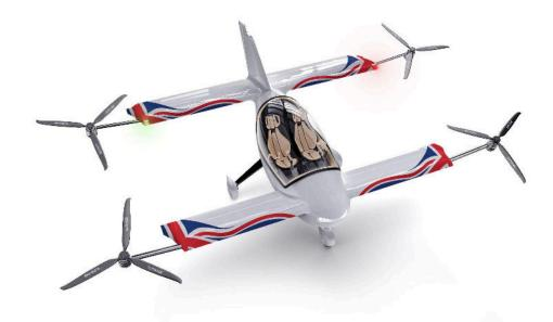
The Axe also offers greatly increased safety compared to a helicopter, thanks to its eight-motor distributed propulsion, each with its own power supply and its glide ability arising from its four wings, which enables power-off landing. Additionally, the Axe is fitted with a ballistic parachute - which a helicopter can never have due to the positioning of its rotors.
